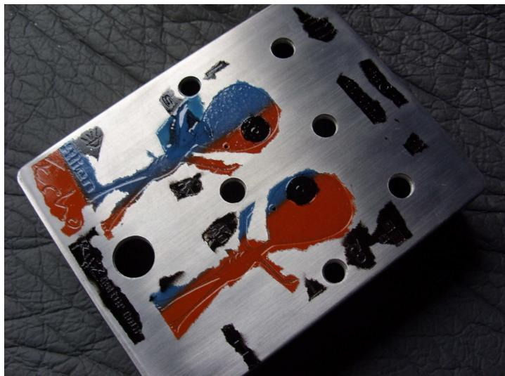
Now remove the paint excess around the designs with 1200 sand paper. Doing it under water will prevent the sanding rests to go into the designs staining the paint.
