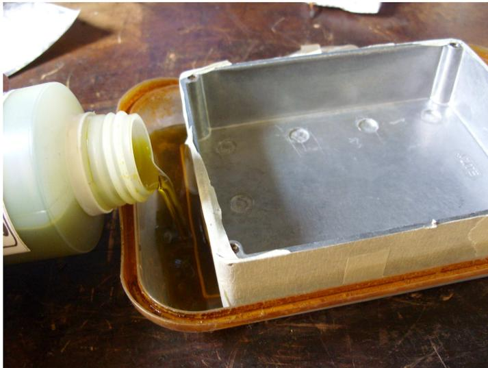
You must be moving the enclosure all the time to remove the metal rests:
