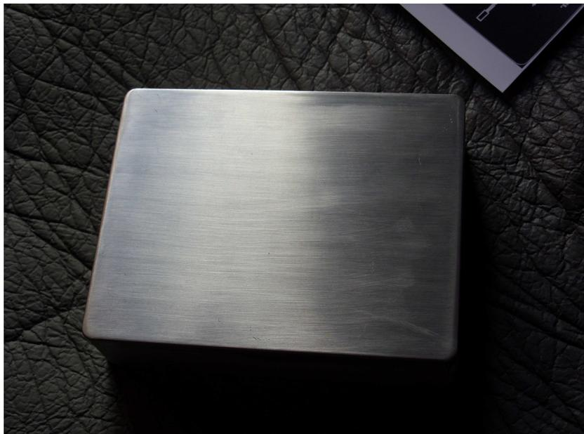
Then you have to dry the enclosure and clear the surface with alcohol to get rid of any rest of metal or dirt.
