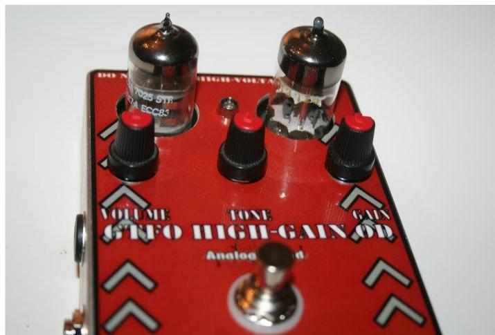
**GTFO is a high gain all tube distortion pedal. Main features:**
