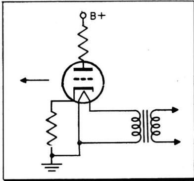
Fig. 6: Class A amp, with grounded heater
