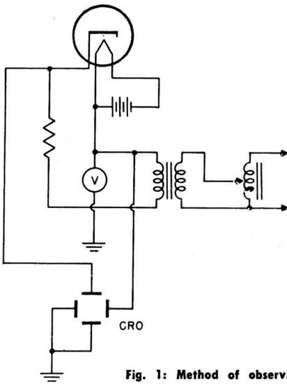
Fig. 1: Method of observing heater-cathode leakage, using an oscilloscope
