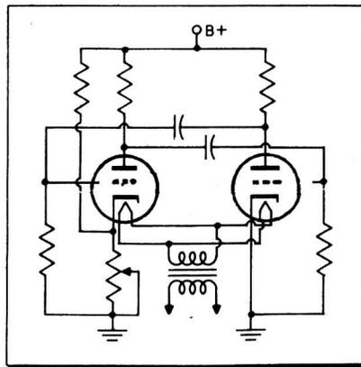
Fig. 8: Voltage divider bias lowers leakage
